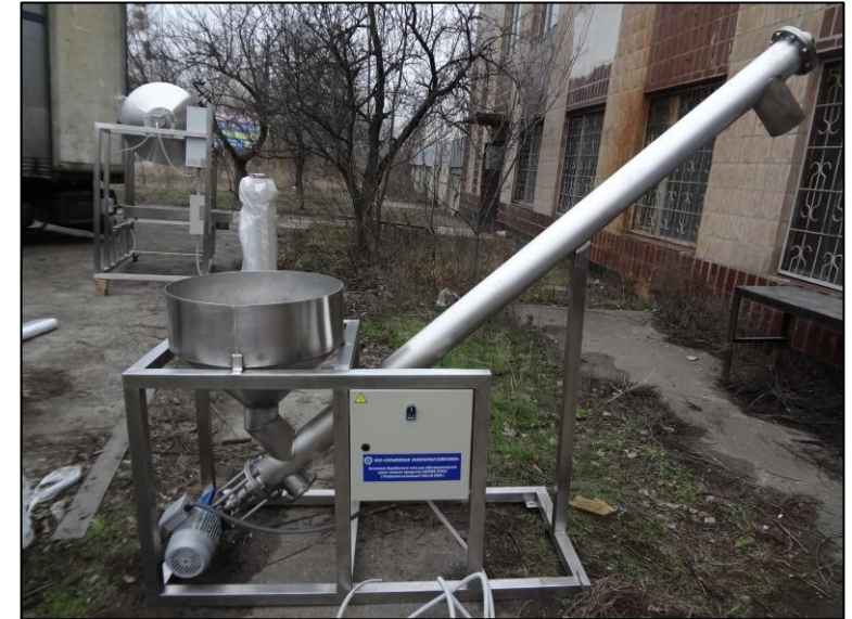
SL screw loader SL120.165ss ( https://www.waterlight.pro/cold-disinfection-in-the-food-industry/stainless-steel-screw-conveyor/ )
